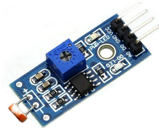
Gambar 2. 11 Modul Photo-Resistor (Sumber : https://bit.ly/4qANiJ9 )
