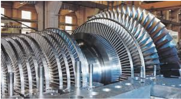
Gambar 3. 3 Sudu – sudu / Blade turbin uap
