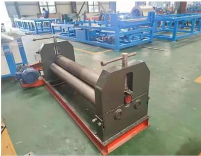
Gambar 2. 9 Mesin Roll bending
