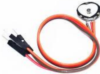
Gambar 2. 5 Sensor Pulse Heart
