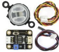
Gambar 2.8 Gravity Analag Turbidity SENO189 Sensor DFRobot Sumber : (Iskandar et al., 2019)
