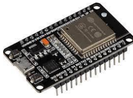
Gambar 2.5 Mikrokontroler ESP32 Sumber : https://docs.zephyrproject.org
