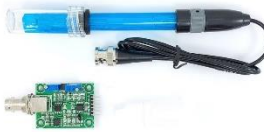
Gambar 2.9 Sensor pH 4502C Sumber : (Wulandari et al., 2024)
