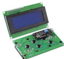
Gambar 2.15 LCD 20x4 I2C Module Sumber : https://uk.robotshop.com
