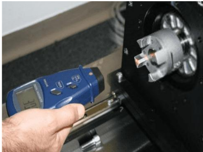
Gambar 2. 10 Non-Contact type Tachometer
