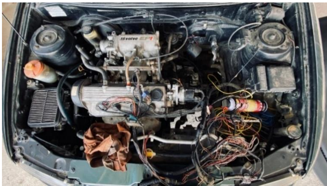
Gambar 4. 3 Restorasi Electrical Wiring
