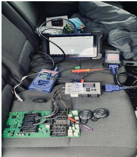
Gambar 3.3 Software Scanner Autel Diagnosis & Programmer Calibration
