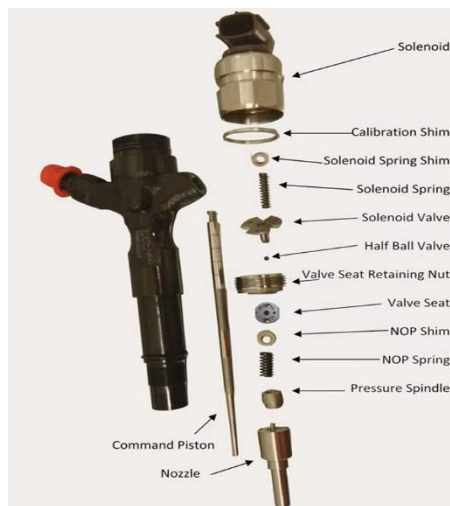
Gambar 4. 8 Assembly Injector Unit Denso
