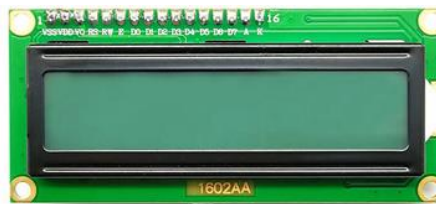
Gambar 2. 4 Liquid Crystal Display 16 x 2
