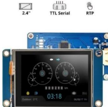
Gambar 2. 3 Nextion 2.4" HMI UART LCD TFT + Touchscreen 320x240 pixel
