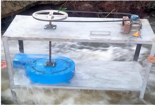
Gambar 4. 1 Instalasi Turbin Kaplan
